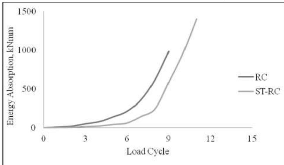
**Figure.4. Variation of cumulative energy absorption capacity with load cycle**
