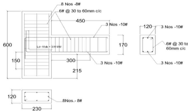
**Figure 3. Reinforcement details of beam-column**
