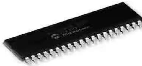
In this system the microcontroller with the specification of PIC 16F877A is used.This is probably the most popular PIC used in many applications because of its low price, high quality and easy of availability.It is ideal for applications such as machine control applications,measurement devices,study purpose,and so on.
