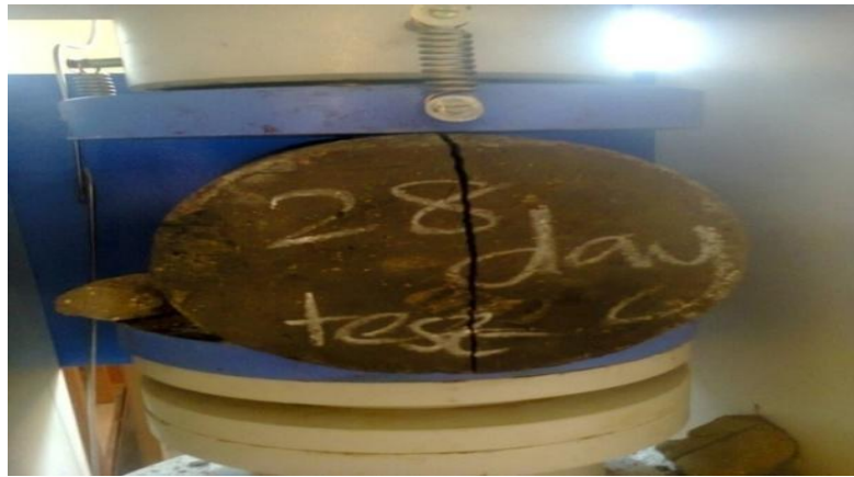
Figure.5.2 Split Tensile Test
