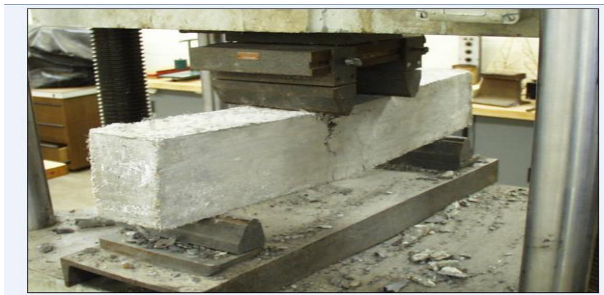
Figure 5.3 Flexural Strength Test
