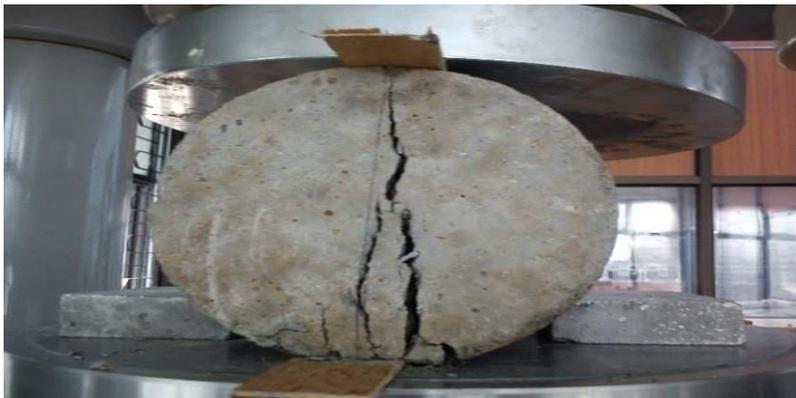
**Fig 3.4 Split Tensile Test Set Up and Failure Pattern of cylinder**
