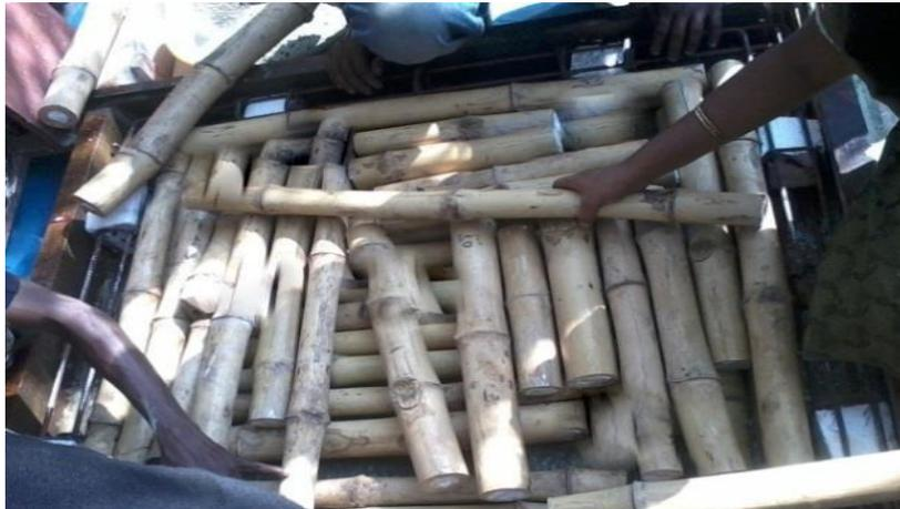
**Fig 4.1 Bamboo As Infill SBA-1**
