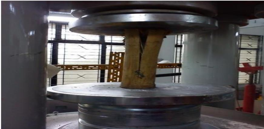
**Fig 2.3 Failure Pattern of hollow bamboo**
