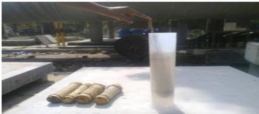
**Fig 2.1 Specific Gravity Test Set Up for Hollow and Strip Bamboo**
