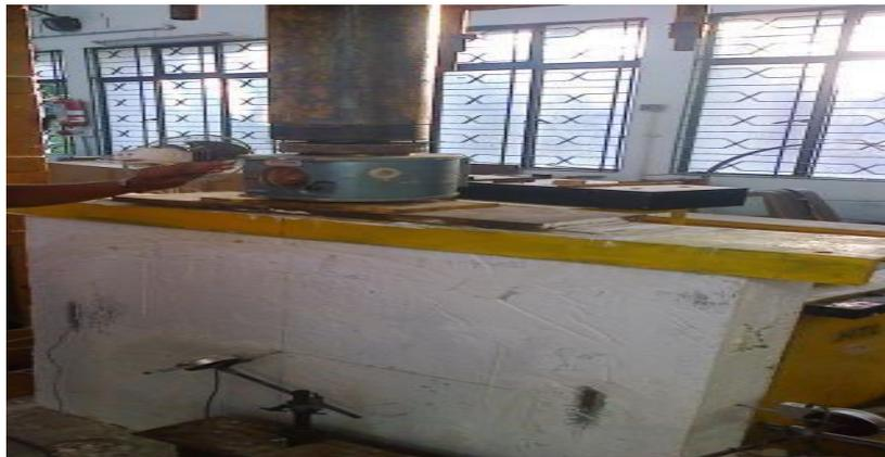
**Fig 4.6 Axial Compression Test Setup with Load Cell**
