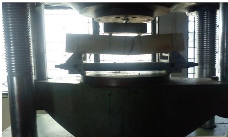
**Fig 3.5 Flexural Strength Test Set Up and Failure Pattern of Prism**
