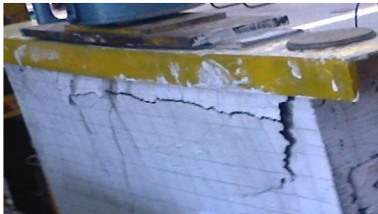
**Fig 4.8 Failure Pattern of SBA-1**
