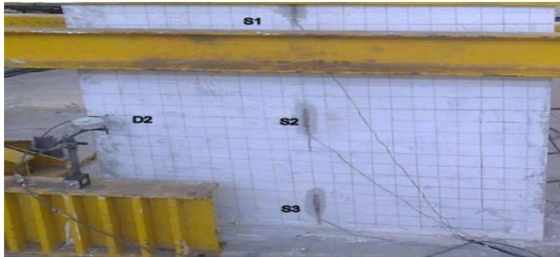
**Fig 4.7 Position Of Strain Gauge And Dial Gauge For Wall Panel SBA-1**
