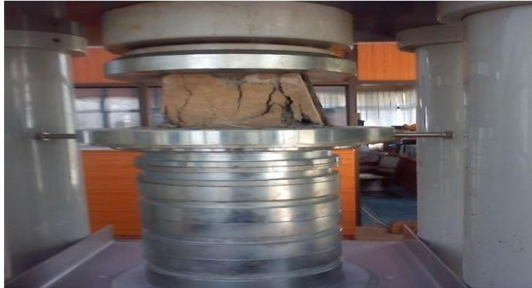
**Fig 3.3 Cube Compression Test**
