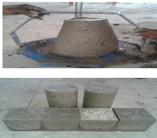
FIGURE: -5.1CASTING OF SPECIMENS
