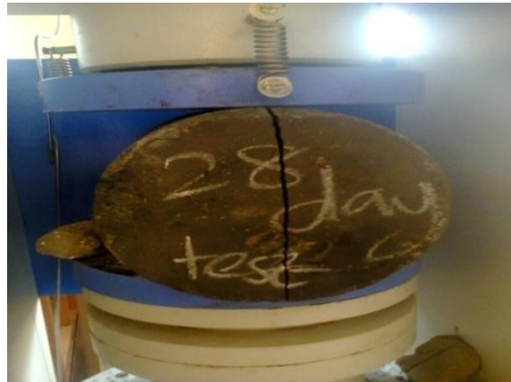
Figure.5.2 Split Tensile Test
