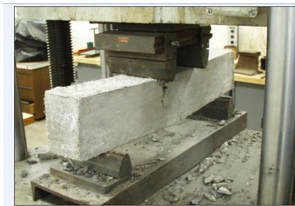
Figure 5.3 Flexural Strength Test
