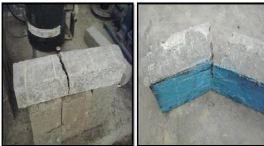
Fig.1.Failure of Plain Concrete
