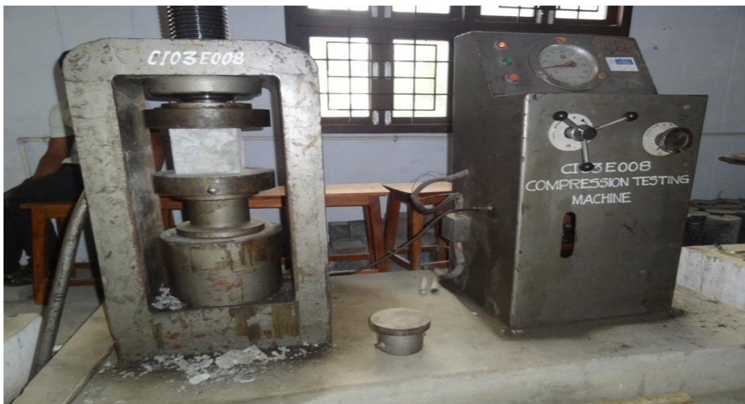
Fig.3. Experimental Setup for Compressive Strength Test
