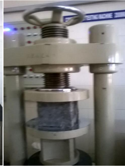
Fig 6 - C.T.M. cube failure
