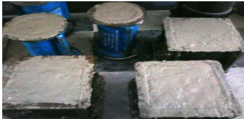
Fig 4 -Placing of mix in moulds
