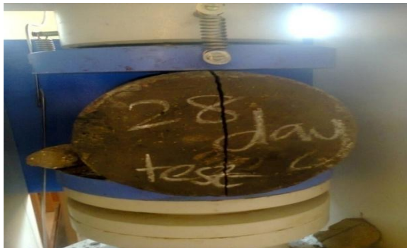
Figure.5.2 Split Tensile Test
