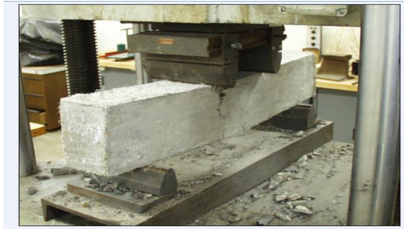
Figure 5.3 Flexural Strength Test
