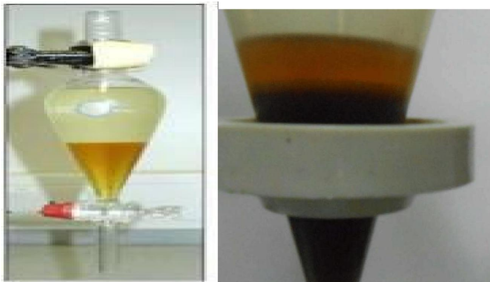
Fig 3 Separation of biodiesel from glycerol
