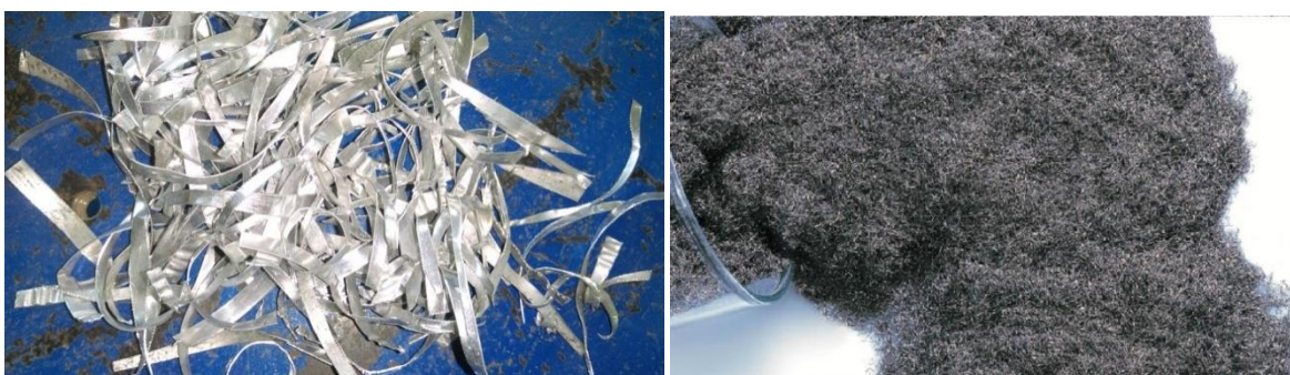
Figure 3: Snapshot for waste tin fibres as well as industrial waste steel fibres
