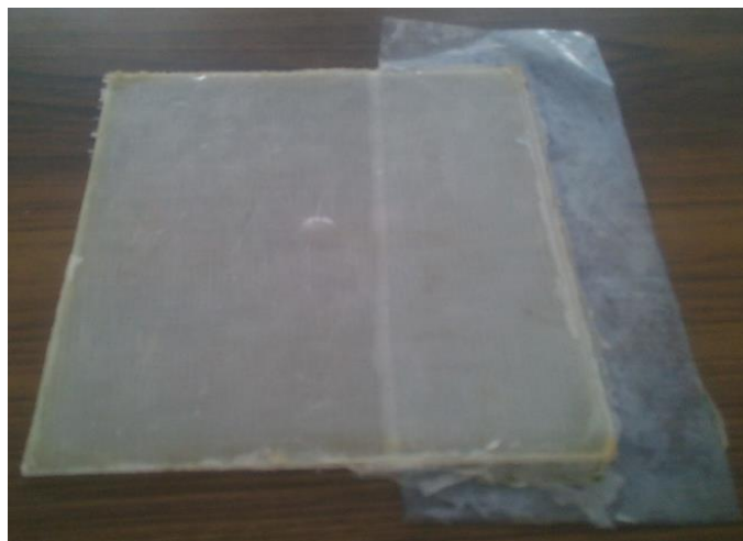
Fig. 1. Prepared GFRP Laminate with Initial Crack
