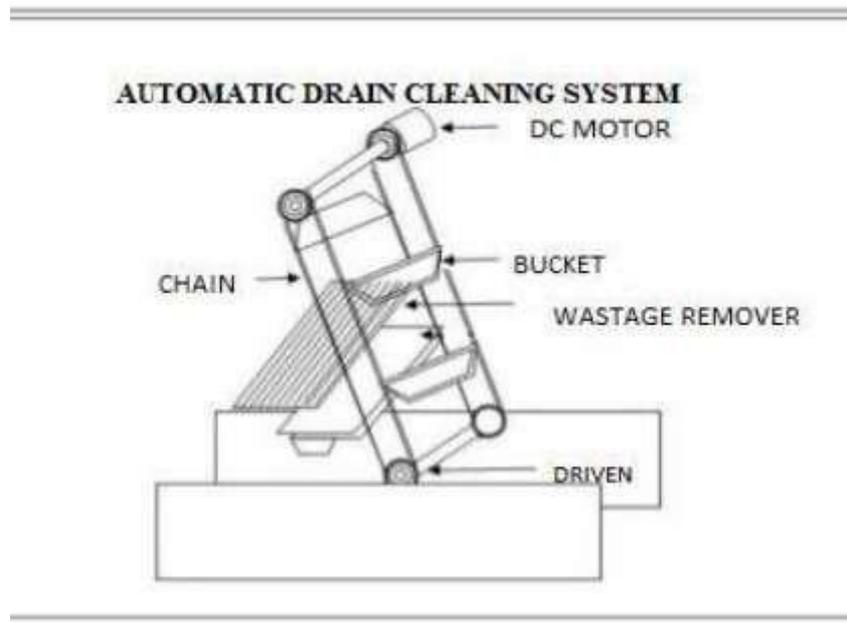
Figure 1: Sketch Diagram of Automatic Drainage Cleaning System
