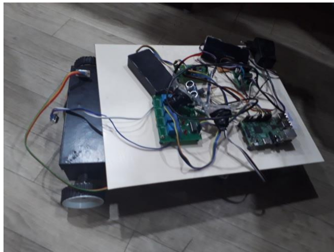
Figure.2 Hardware snapshot for an Robotic-Wheelchair Control Head Orientation and Eye Ball Movement Control with Health Monitor System
