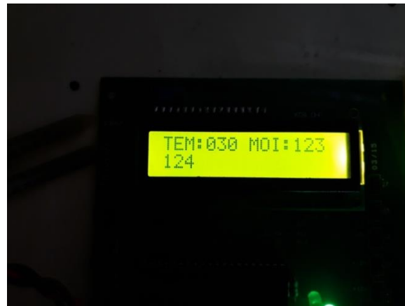
Figure.4 Hardware output snapshot of the LCD display the temperature and moisture level of the soil with help of sensors
