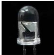
An IR light-emitting diode (LED) is a semiconductor diode that emits incoherent narrow-spectrum light when electrically biased in the forward direction of the p-n junction, as in the common LED circuit. This effect is a form of electroluminescence.
