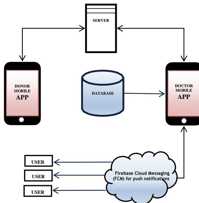
Fig 5.1 System Architecture
