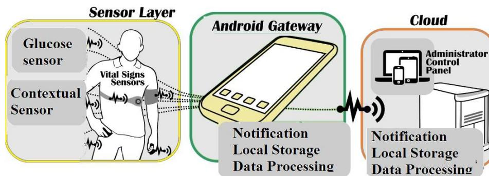
Fig. 3.2: Continuous Glucose Monitoring using IoT
