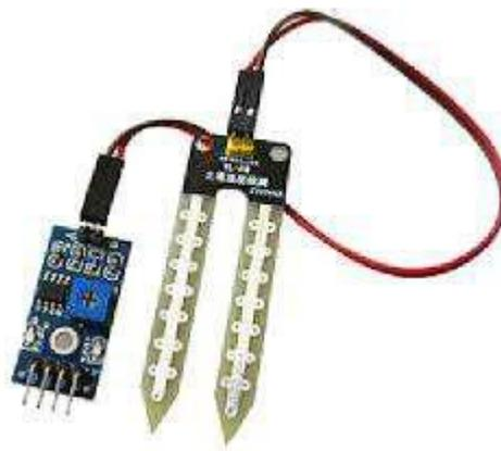
**Fig 4.5: Soil Moisture Sensor**
