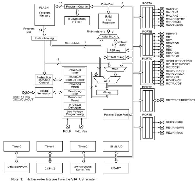
Fig 4.1 : Architecture of PIC16F877
