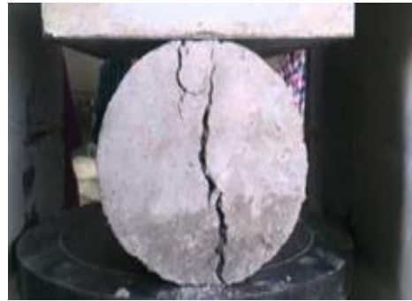
Fig.4 shows the split tensile strength of concrete using Glass powder and Bagasse ash at 28th day.
