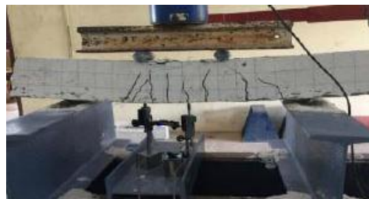
Figure 5 shows the load and the beam made with S4 mix
