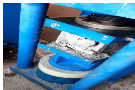
Fig.5.1 Compressive Strength Test
