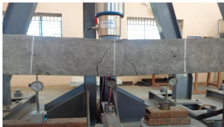
FIG.5.4 LOADING FRAME TEST SETUP
