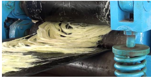
Fig. 2.4 Sisal Fiber Extraction
