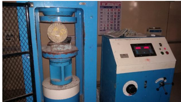
Split tensile strength test setup
