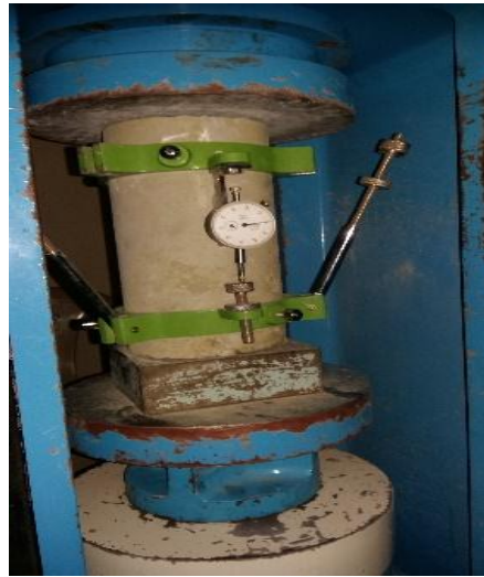
Testing setup for stress – strain relationship
