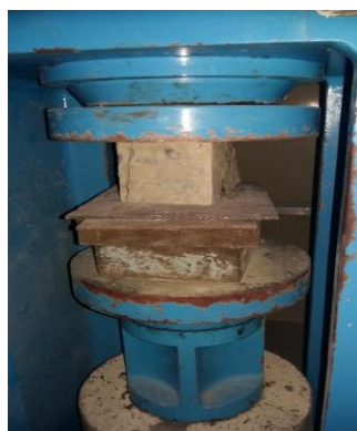
COMPRESSIVE STRENGTH TEST SETUP
