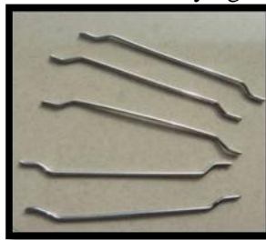
Shows the hook end steel fiber of 50mm length
