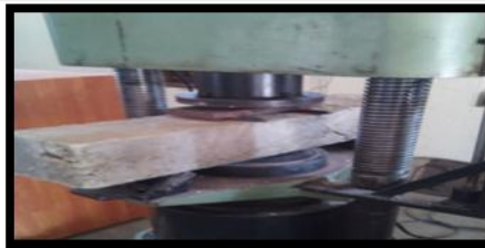
Shoes test setup of slab panel
