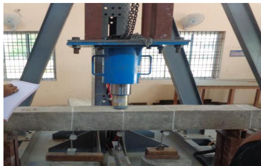
FIG.5.4 LOADING FRAME TEST SETUP
