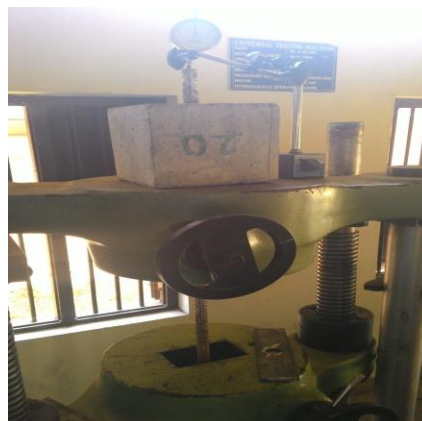
Arrangement of pullout test in UTM machine
