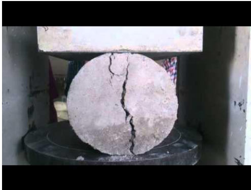
FIGURE 2: Split tensile test
