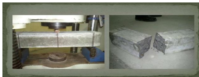
FIGURE 4: Flexural strength of beams
