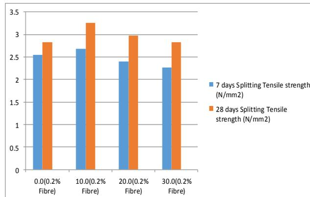
**Fig.Effect of silica on splitting strength using OPC:**
