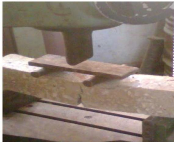
**Fig. Determination of Flexural strength of prism**
