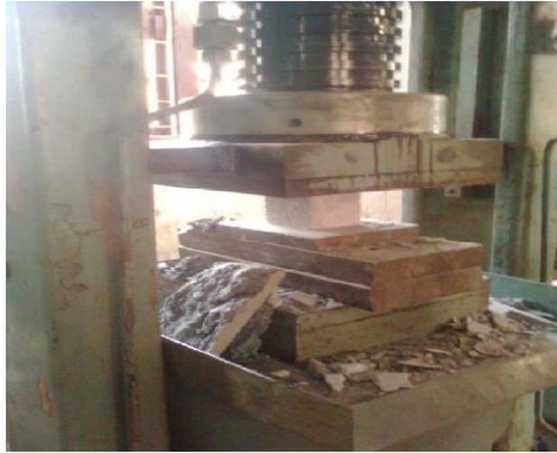
**Determination of splitting tensile strength of cylinder**
