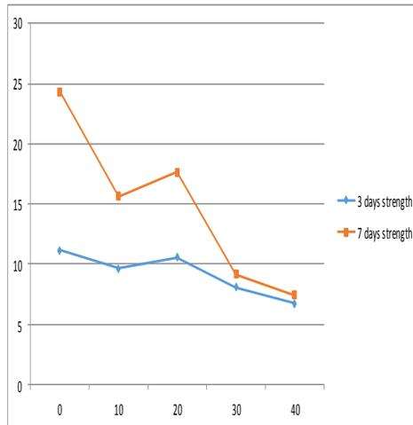
Fig.4.4 Variation of Compressive strength of mortar with different SF %
